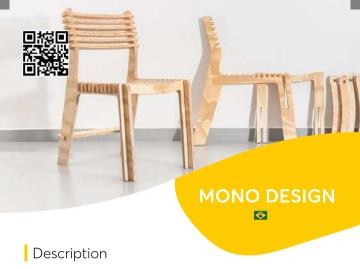
Mono Design designs furniture tailored to users, which is always produced through digital fabrication. Using CNC Router technology, digital files can be shared with its producers around the world, so that the pieces are manufactured as close to the user as possible.
