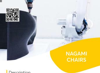
The Nagami company invests in overcoming the limitations of conventional design. To achieve greater efficiency, the company developed its own extrusion method for additive manufacturing, making its line of chairs rich in details and sinuous lines that bring exclusivity to its customers.
